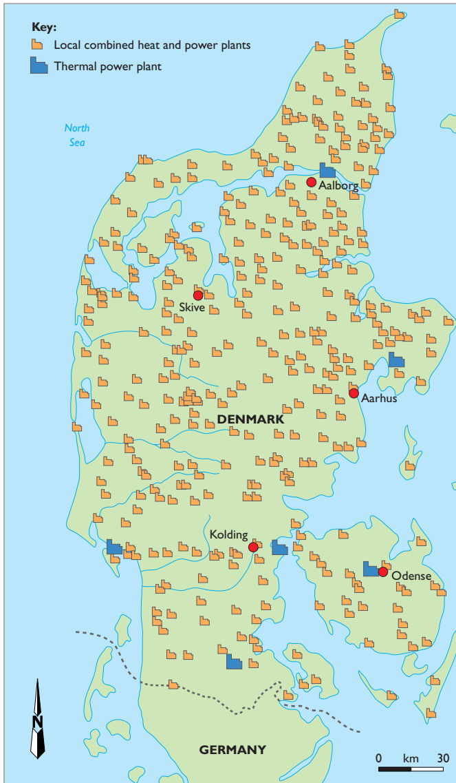
Fig. 2. West Denmark's six thermal power stations of 3516 MW are supplemented by a further 1450 MW from combined heat and power plants in most towns and villages
